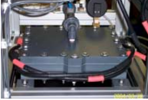
Figure 3. The capacitor cell
